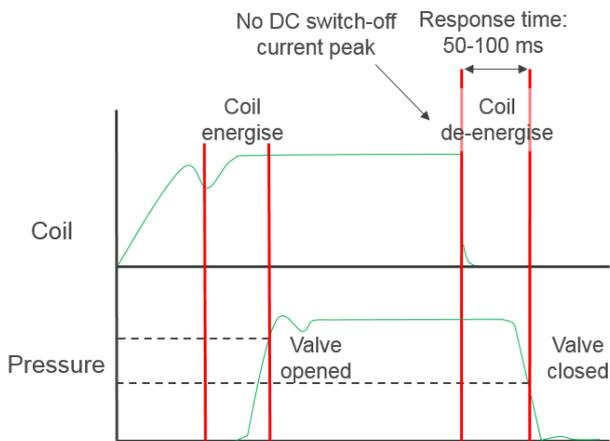
Figure 3: A fast closing solenoid valve increases the safety of your application
