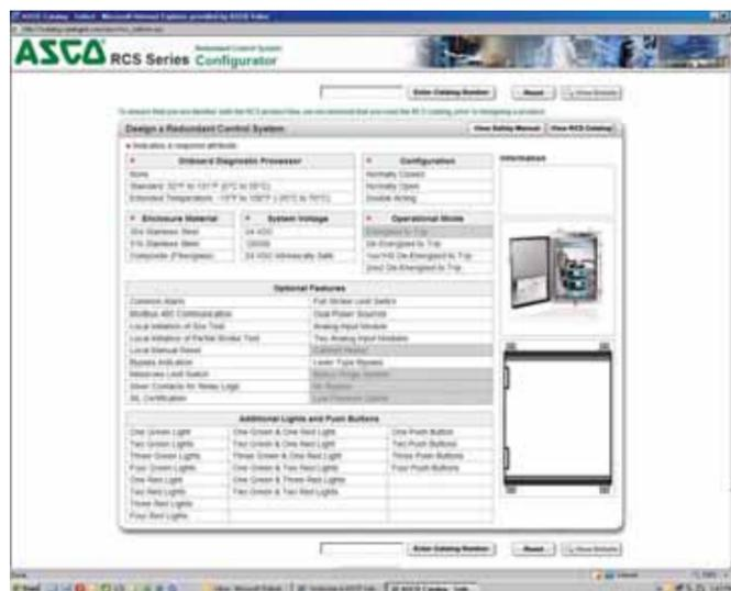
Online specification tools, such as ASCO's Redundant Control System (RCS) configurator (pictured here), allow users to build virtual valve assemblies with a variety of options, including diagnostics capability, materials, manual resets, and SIL ratings. Such tools are designed to enable specifying engineers to more quickly and accurately select the valve solution that is most appropriate for a given application.
